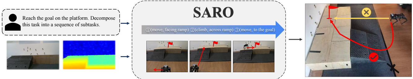
Fig. 1: SARO achieves space-aware navigation capability for 3D terrain crossing. Our system utilizes the reasoning and motion planning ability of the VLM model, with a design of task decomposition and a closed-loop sub-task execution module. While traditional navigation approaches (yellow) fail in reasoning 3D environment, our system (red) guides the quadruped robot to cross the accessible intermediation towards the goal.
